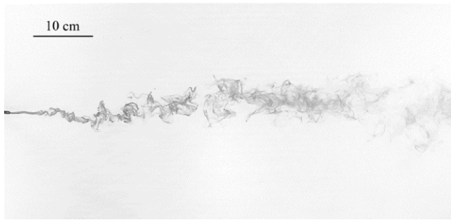
Figure 1. Flow visualization of the chemical plume, which is created via a continuous iso-kinetic release of a dye solution into a fully developed turbulent boundary layer. The view is from above, with the flow moving from left to right.
